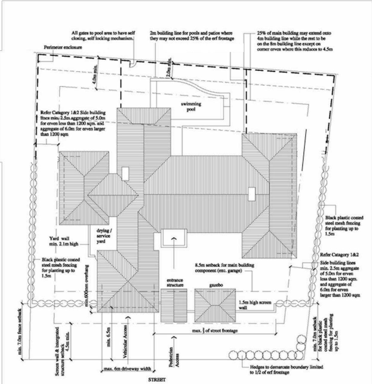
**ILLUSTRATION OF TYPICAL RESIDENTIAL UNIT WITH REFERENCE TO BUILDING LINE, YARD WALLS, SCREEN WALLS AND FENCE ENCLOSURE.**
